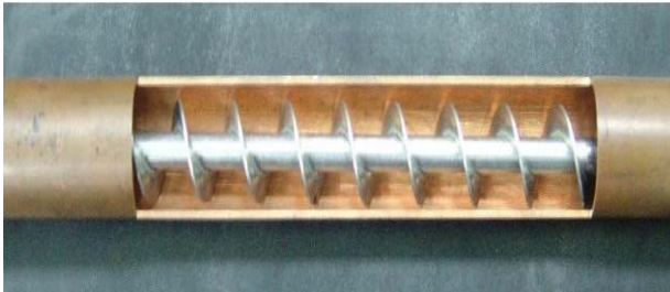
FIGURE 1: The inner tube fitted with the full-length helical tape.
